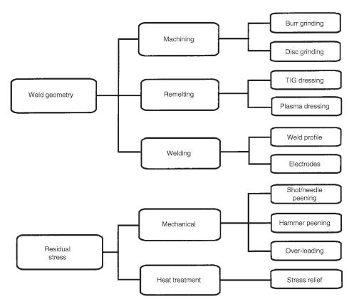
$\pmb{Fig.~24} \quad \text{Range of postweld fatigue life improvement techniques. TIG, tungsten inert gas. Source: Ref 16}$
